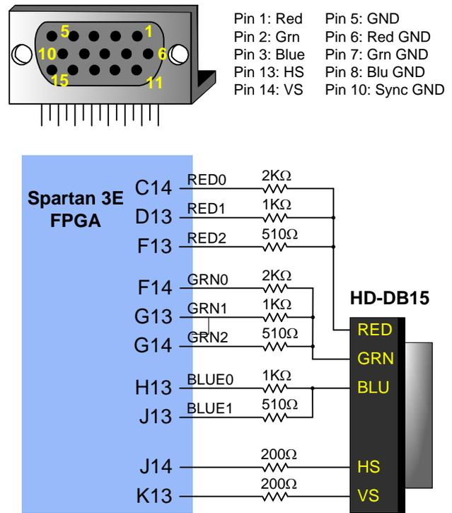
Figure 13. VGA pin definitions and Basys2 circuit
